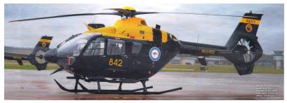
with winches/hoists and a hook for underslung loads and can carry six people, although in the training role it will be limited to four people. During training an Instructor will sit in the left seat with the Trainee in the right seat. The EC135 is an electronic-age helicopter with digital displays and dual certified GPS navigation system, allowing flight in cloud with no requirement for ground-based navigation systems.
